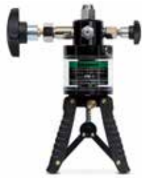
Beamex PGHH 校准泵 0 ... 700 bar / 0 ... 10,000 psi
